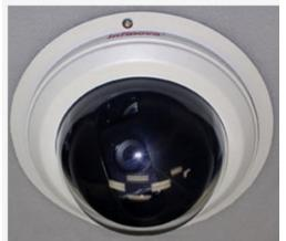
camera is ideally suited for parking lots, garages, filling stations and similar installations. The V1740/C has Anti-ice/anti-mist, built-in heater and air circulatory system included.
