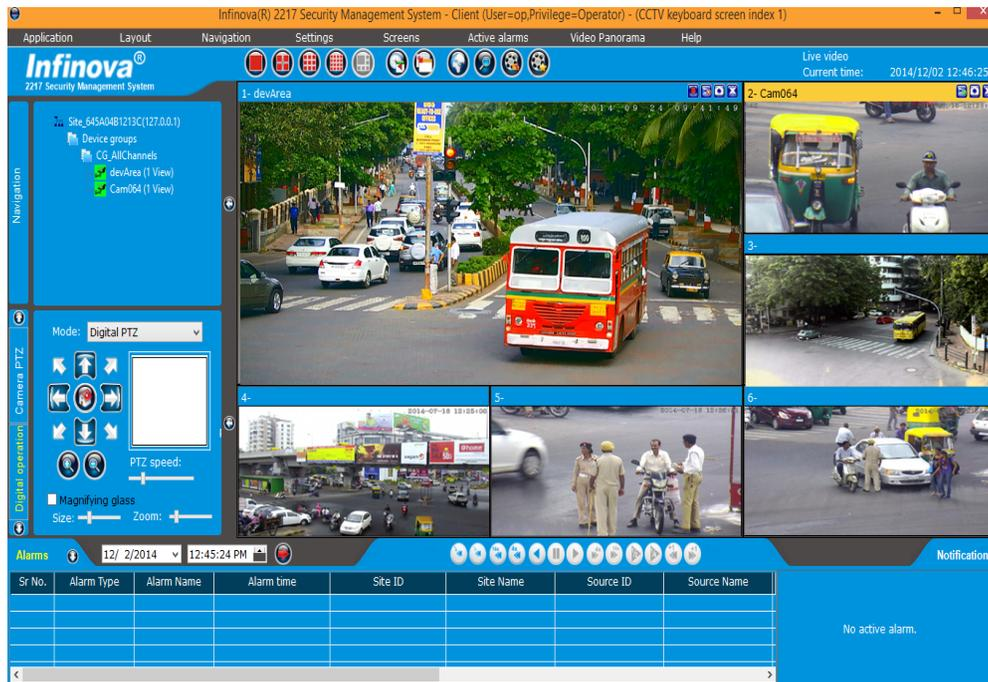
Video management software (VMS) is vital for any surveillance system. It is designed for managing cameras and recording settings. Through VMS, you can view multiple camera feeds and also set alerts for motion detection and tampering. It enables you to review and analyze recorded videos, helping you keep your residential or commercial facility safe.
