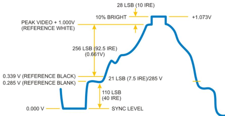
Now, let's review the IRE value. The lower the IRE value, the darker the black areas are, while the higher the number, the lighter they are. Generally speaking, the IRE value expresses the video signal amplitude. A video signal is useless when lower than 25 IRE (175 mV) since the video displayed on the monitor will be totally dark. Therefore, the IRE value is most often described as a number above 25, generally around 30 and, sometimes, as high as 50.
